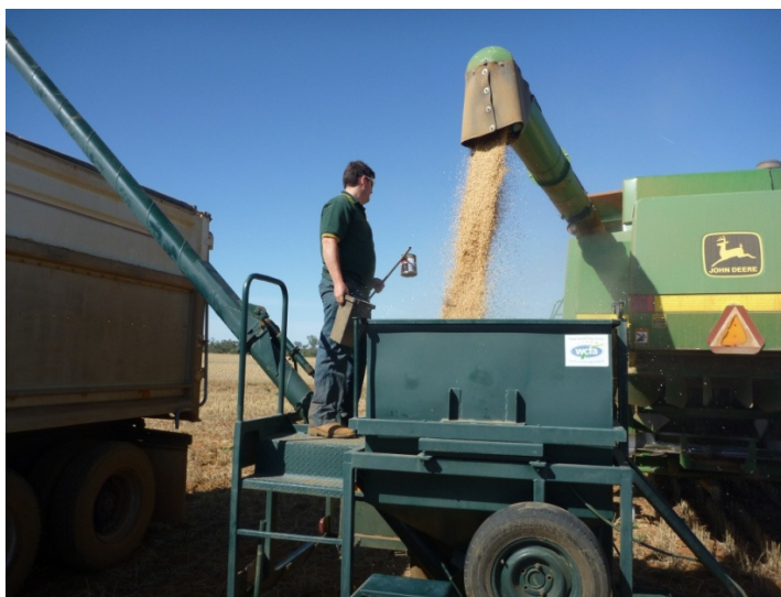
Plate 2. Measuring grain yield from a commercial harvester using a weigh bin
